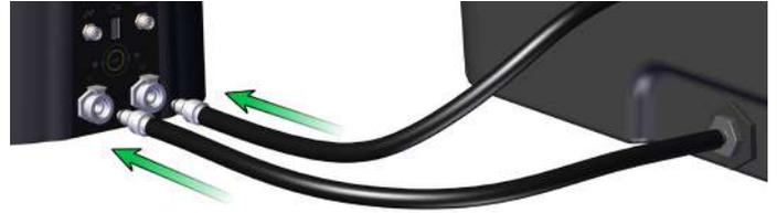
**10.** Connect the level/temperature probe cable.
