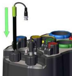
**6.** Insert the pH probe as far as it will go and tighten the probe clamp.
