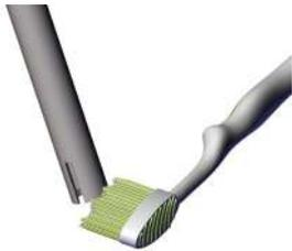
**3.** Clean the EC probe with the supplied brush.
