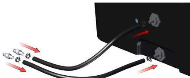
**9.** Connect the tub supply tubes to the NIDO ONE V2 as follows: Tub OUT tube to NIDO ONE V2 IN input and Tub IN tube to NIDO ONE V2 OUT input.
