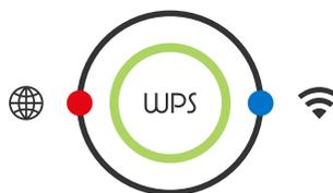
If the blue light is flashing, it indicates no internet connection. In this case, it is necessary to check the router for firewall blockages.
