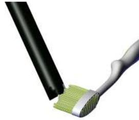
**4.** Clean the pH probe with the supplied brush, avoiding touching the glass bulb with your fingers.
