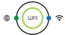
If the left light is red, move the access point a few metres away from the NIDO ONE V2, making sure there are no walls or obstacles between the NIDO ONE V2 and the access point.
