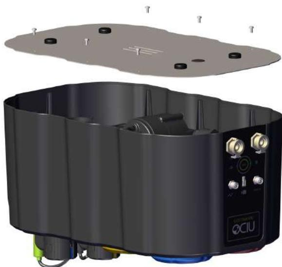
**2.** Remove the black cap located on the steel plate and use the resulting opening to pass the RJ45 network cable through.
