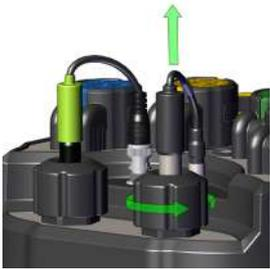
**2.** Pull out the EC probe by unscrewing the probe gland.
