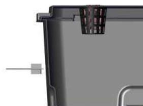
Drill the water inlet hole at a point above the maximum water level.
