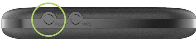
4. Press the WPS button on the NIDO ONE V2 for 12-15 seconds, or until the blue light on the left side starts flashing.
