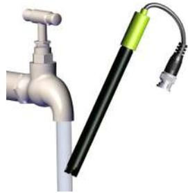
**5.** Wash the pH probe under running water and dry the outside with a clean cloth.
