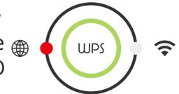
If the left light is green and the right light is flashing blue, NIDO ONE V2 is connected to its access point, but no Internet is available.
