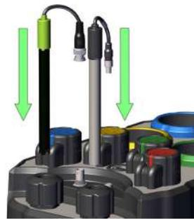
**3.** Insert the pH and EC probes into the probe clamps until they are flush. Screw in the probe clamps with light force and connect the appropriate connectors.
