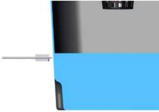
Drill the hole for the level probe (11mm diameter tip) with the centre of the hole where you want the ALERT water level to be.
