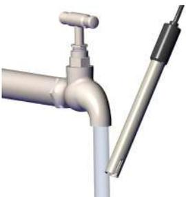
**4.** Wash the EC probe under running water and dry the outside with a clean cloth.
