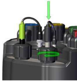
**5.** Insert the EC probe as far as it will go and tighten the probe gland.
