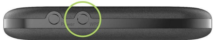
6. Wait approximately 30 seconds for the pairing to complete. This is indicated by both blue lights on the side panel of the NIDO ONE V2 flashing intermittently. Next, restart the NIDO ONE V2.
